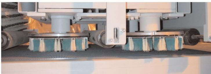
Additional hold down roller between discs for better transport of small work pieces even without vacuum
